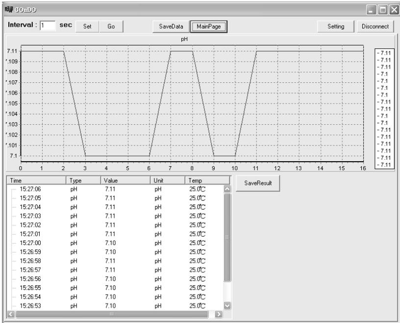
7. Click **SaveData** and then press and hold **STO/RCL** to enter Recall mode. Press **MODE** to export all the records to the program. The records can also be saved as a .txt file by clicking **SaveResult** in this window.
